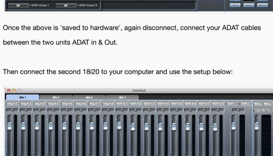
Once the above is 'saved to hardware', again disconnect, connect your ADAT cables between the two units ADAT in & Out.
