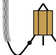
Inner, black cloth wire is the hot output. It connects to the 3-way switch
