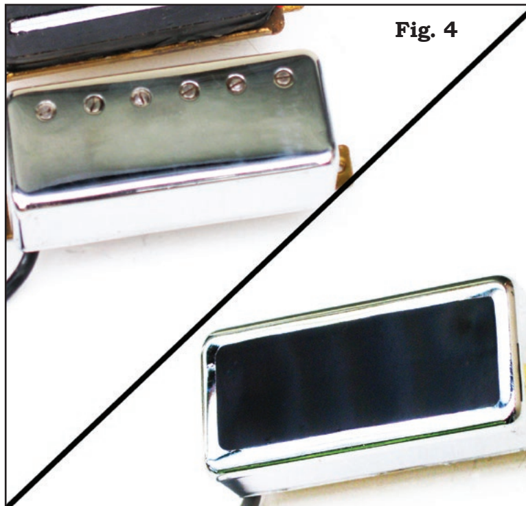
Fig.4. Epiphone mini humbucker: A: original with and without brass cover. B: modified (top opened, embedded in epoxy resin)
