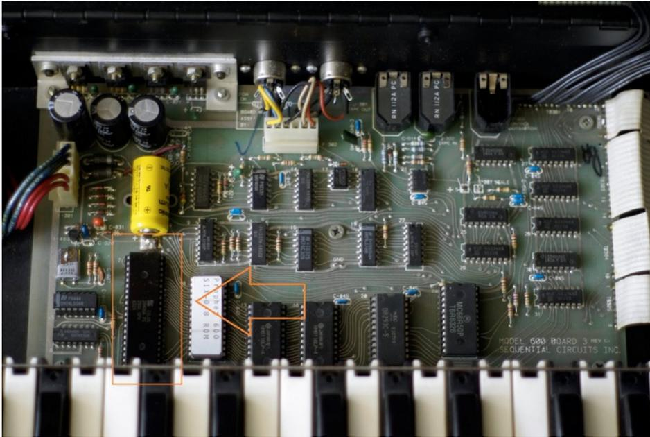
3. Locate the Z80 microprocessor on the lower left hand corner of the computer board and carefully remove it using an IC extractor or nudging it up on each side until it is loose enough to pull off of the socket. Store it in a safe place on conductive foam.
