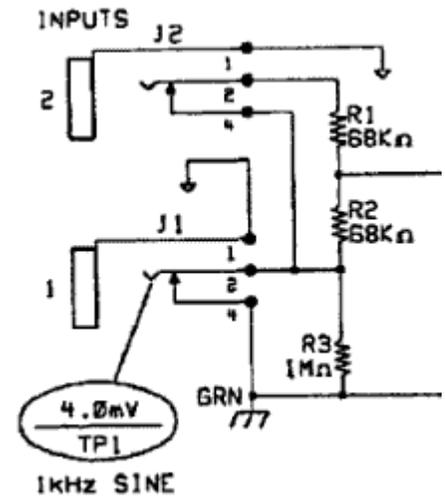
**7a.** If you're using a **closed-circuit mono jack**, keep reading. If not, skip this step.
