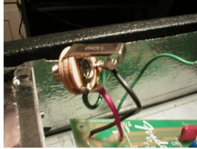
Input 1: Here we can clearly see the green jumper wire between shorting lug and ground lug. If we look in the background of the first picture, we can see where I didn't unscrew the ground wire (long green wire) and it broke while I was soldering. DOH! That's something else you should do. I'll have to resolder it back into place before I do testing later.
