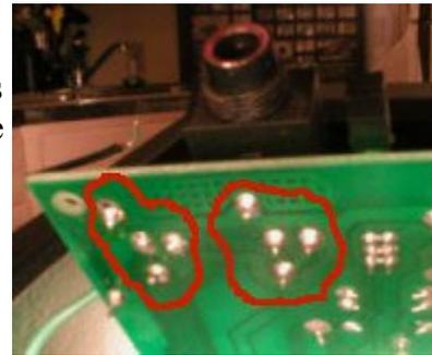
Now that we've removed a plastic jack, look at the bottom of it. Four lugs should be coming out of holes on the bottom. These lugs should have numbers above them. In this case they should be 1, 4, 5, and 2. NOTE: To get a better view, click the picture to the right to enlarge it.
