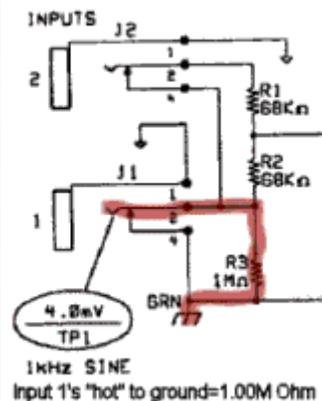
Here is a pictured example of the first reading on the chart: 0.98M $\Omega$  is "close enough" to 1.0M $\Omega$ .
