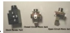
**Important info for Switchcraft users:** The positioning of the lugs on the Switchcraft and the Radioshack jacks are NOT the same. The Switchcraft's "2" and "4" lugs are
