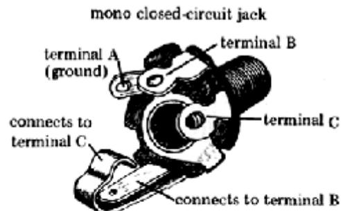
with plug not inserted, terminals B and C short together
