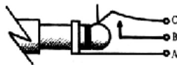
Here's a little diagram/schematic of the closed-circuit (sometimes called a "shorting jack"). Hopefully it'll help you better understand how it works.
