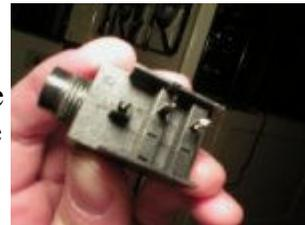
**5.** After deciding which brand of jack to use (Switchcraft or Radioshack), we must now decide which *type* of jack we're going to use. The most ideal type is a **closed-circuit** mono jack—also called a "shorting jack." (The Switchcrafts from Mouser are this type.) It has three lugs and physically performs the same action as the plastic jack we're replacing. Logically, we can assume the plastic jack is also "closed-circuit."
