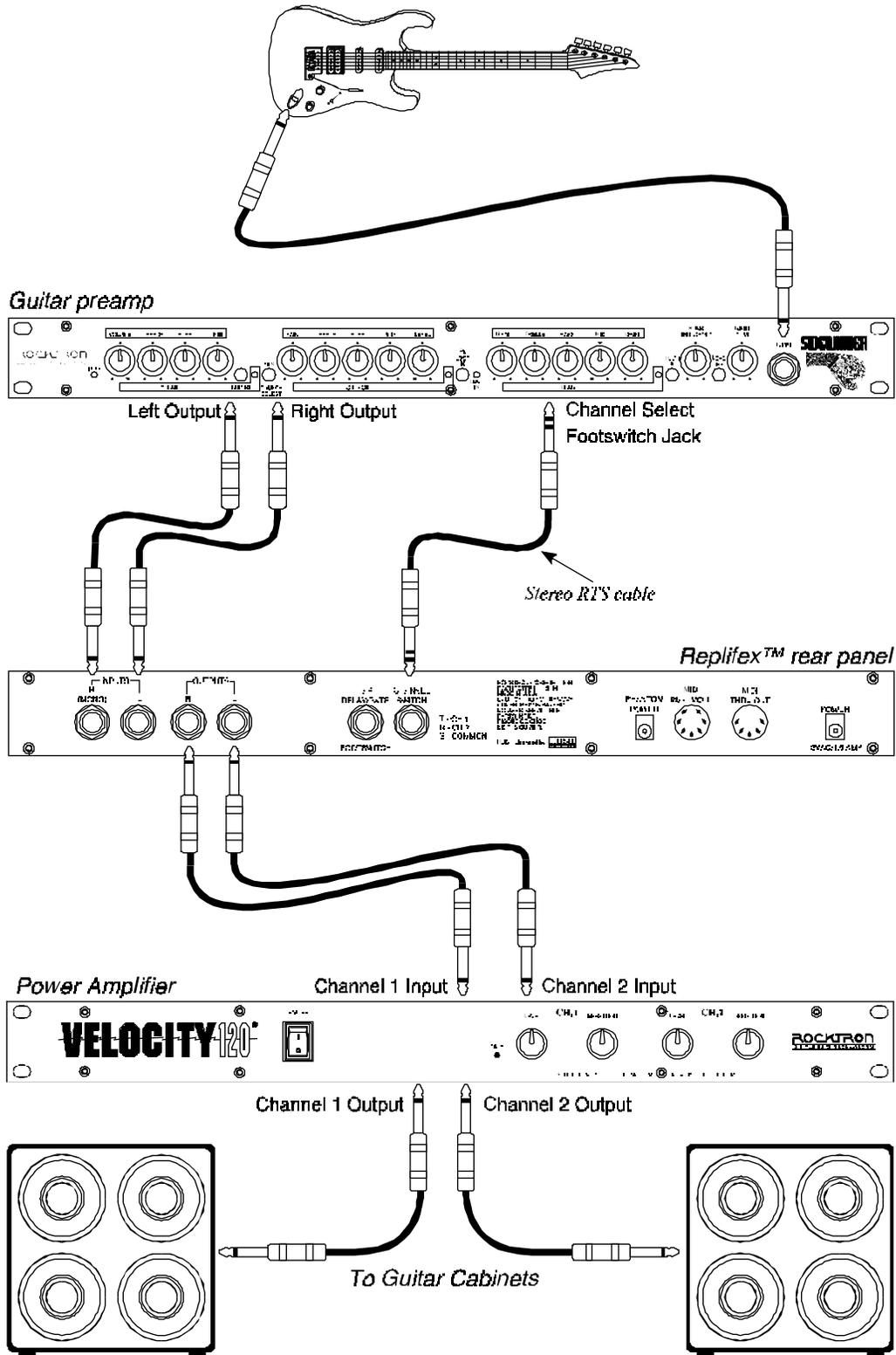
Using the Replifex™ in a preamp effects loop
